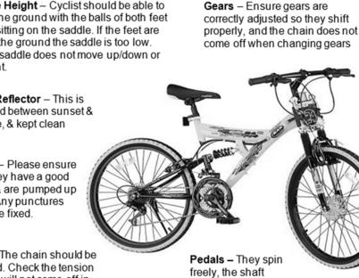
Headset - Check for "Shake" by lifting bike off the ground. If the frame moves or rattles before the front wheel then the headset needs tightening
